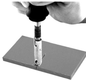
Tacking plastic parts with stitching action
