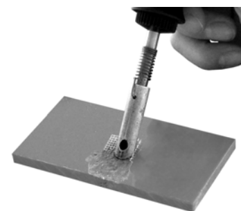
Cover the mesh with melted plastic
