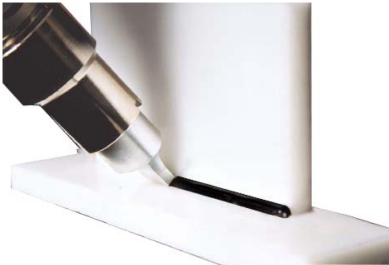
Fig. 4a: fillet weld using the welding tip T 200001.
