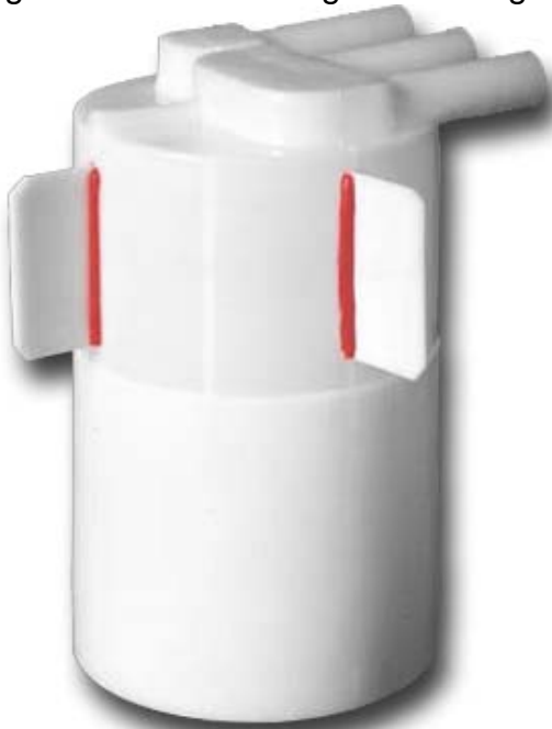
Fig. 4a: fillet weld using the welding tip T 200001.
